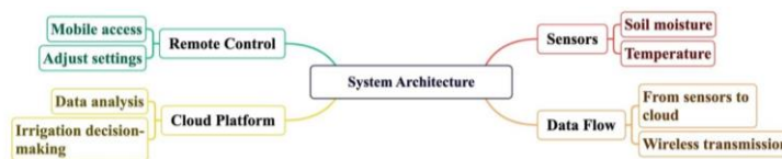
Figure 3: Illustration of an IoT-based smart irrigation system architecture
