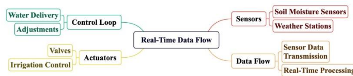
Figure 3: Real-time data flow in an IoT-based irrigation system, from sensor to actuator.
