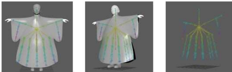
Figure 4: Glove Puppet Skeleton with Dynamic Joint Chain.
